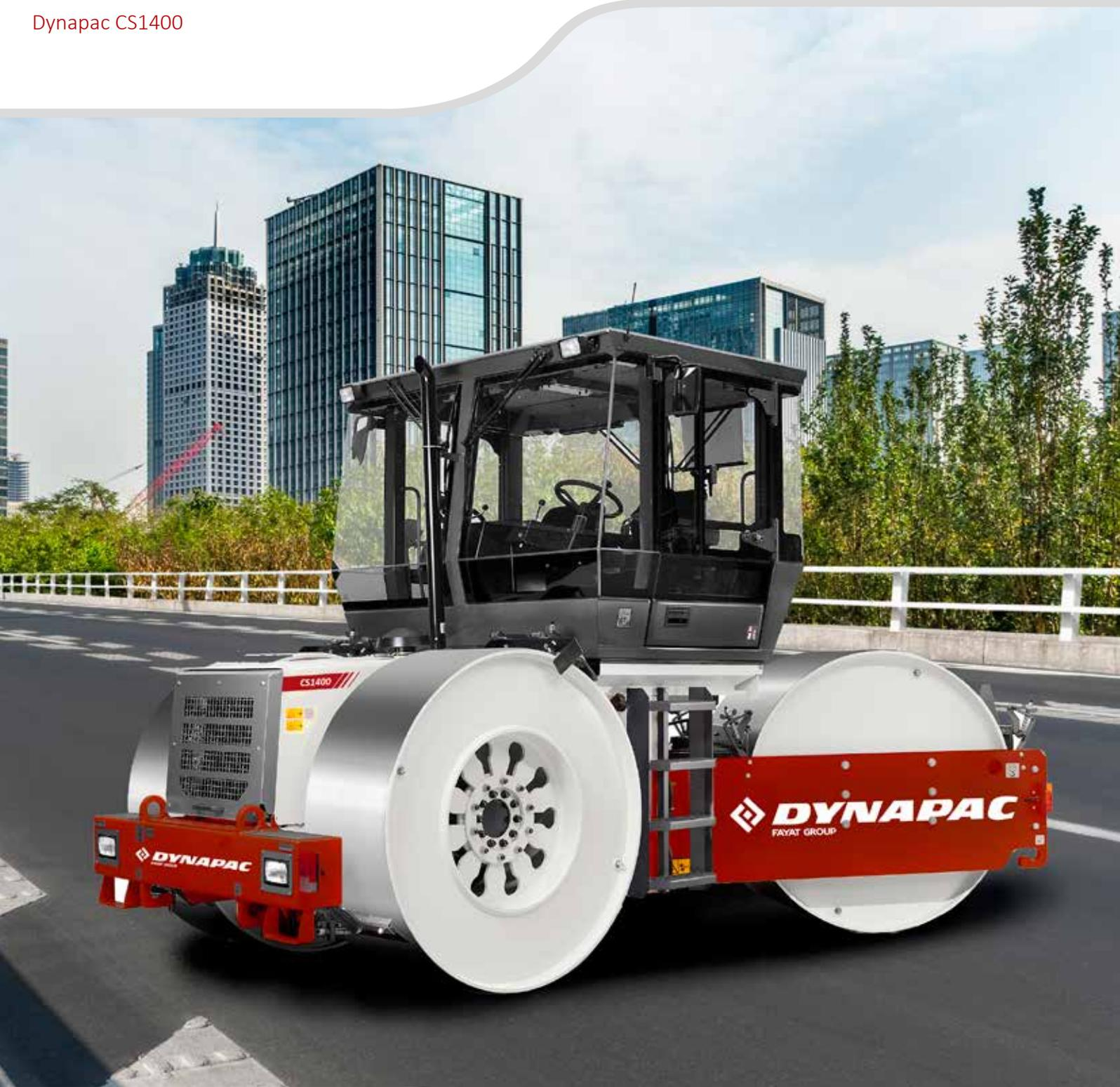
**THE DYNAPAC CS1400 STATIC ROLLER** is a modern, articulated three-drum roller with the same static linear load and drum diameter on all drums. The roller covers the asphalt mat with its full width. The CS1400 roller is used primarily to compact asphalt when the course has a typical thickness of up to 50 mm, depending on the stiffness of the asphalt compound and the prevailing weather conditions.
